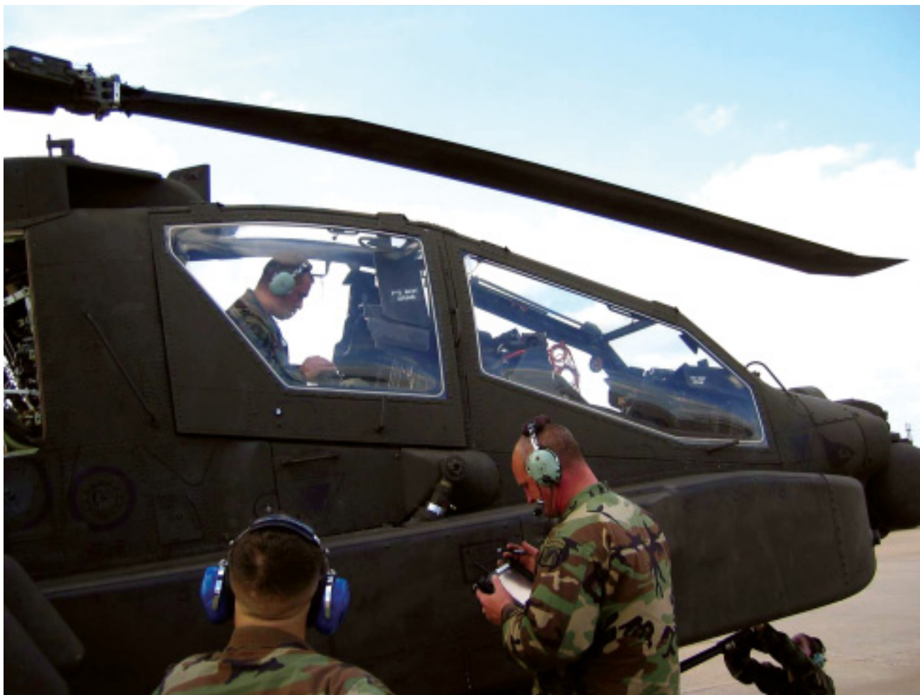
An Apache Maintenance crew performs an 'After Maintenance Operational Check.' An Air Force mechanic on the ground equipped with an Atigo® T High Bright and communications headphones runs through an operational safety check list with a mechanic in the cockpit. MRO software developers such as MIRO Technologies are leading the way in developing new applications to benefit defence logistics
