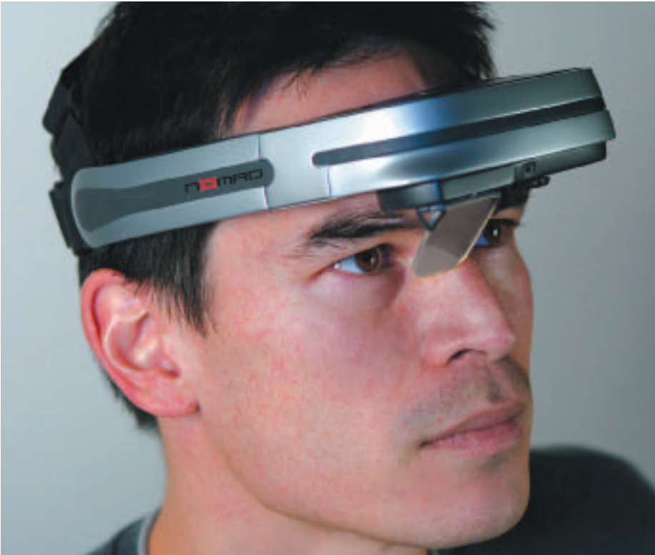
Weighing only 4.5 ounces, the Nomad head-worn Display Module can either be mounted under the brim of a cap or integrated into a headband.
